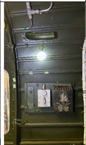
The Navigator's Communications and Flight Suit Heater Control Mounting Plate has been refurbished and re-installed.
