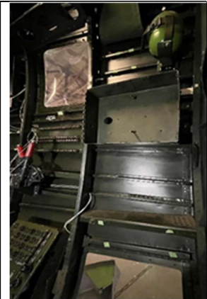
The forward compartment Bombardier's Panel has been relocated to its correct place so the Navigator's Panel and Intervalometer can be positioned.
