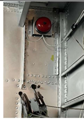
The Bomb Bay Bail-out Bell has been refurbished and re-fitted at the aft portside bulkhead.
